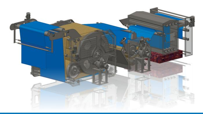
Confine Shrinking range improves finishing process of woven and denim fabrics by allowing necessary shrinkage and stabilization of the fabric.
